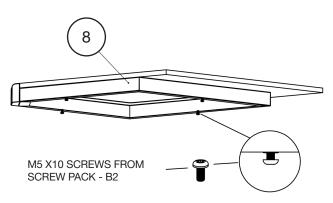
Partially install the M5x10 bolts into the Top Module assembly, leaving them loose for the following step.
