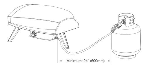
Only use the appliance with gas cylinder that does not exceed 600mm in height and 300mm in diameter.
