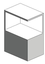
In the case of balconies, at least 20% of the total of the side, back and front wall areas shall be and remain open and unrestricted.
