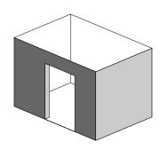
An enclosure with walls on all sides but at least one permanent opening at ground level
