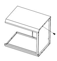
3. Position the front top bar and secure with the 4 screws. Position the top plate and secure with the 6 screws.
