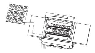
12. Install the splatter plate to the inside of the BBQ.
