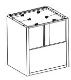
4. Tip assembly upside down and position the 2 caster alignment plate then secure with 2 screws per plate. Position the lockable caster wheels at the rear and secure with 4 screws each. Position the remaining caster wheels at the front and secure with 4 screws each.
