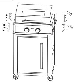
10. Install the side tables to the brackets and secure with screws 2 per each side.
