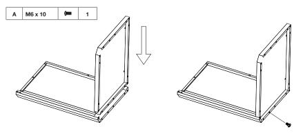
2. Position the back panel and secure with the 4 screws. Position the right side panel into place and secure with the screw.
