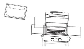
13. Install the grill and plate on the top surface of the splatter plate.
